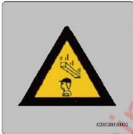
Warning: Pay attention to falling article! Please wear the safety helmet!
