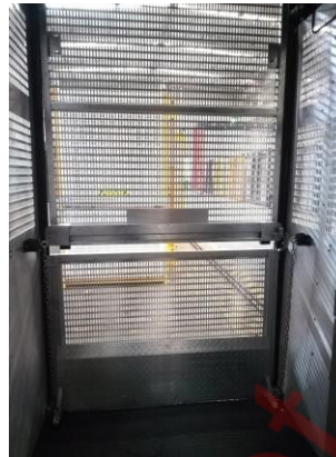
(d) Exit door combined with little manual operated load ramp inside cage
