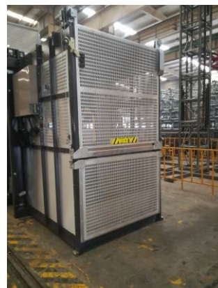
(b) Exit door with double opening
